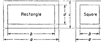
Nominal dimension *a* determines tolerance applicable to both *a* and *c*.
